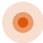
FIBRE MULTIMODE 62.5/125 µm - OM1
